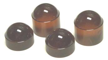
Figure 6. Lenses produced using HRDT
